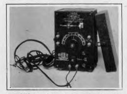
THIS crystal receiver was designed to cover a wave-length range of 170 to 2,650 meters. The set is sold complete with a pair of sensitive telephone receivers.
