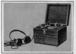
RADIOLA SR. is designed to fill the popular demand for an inexpensive set for broadcast reception with a greater range than a crystal set. Radiola Sr. makes use of the Regenerative Circuit in conjunction with a vacuum tube detector. A big feature of Radiola Sr. is that the filament of the vacuum tube may be operated from a single dry cell.
