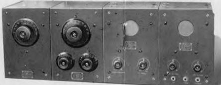
R ADIOLA Super Selective Combination consists of Models RT primary coupler; RA secondary coupler; AR 3 stage radio frequency unit, and DA detector, 2 stage audio amplifier illustrated, in the order given, at the head of these pages. It is designed for use with an outdoor antenna for broadcast reception over long distances, and under conditions where extreme selectivity is desired.
