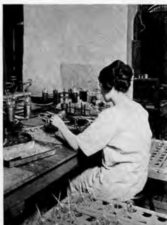
Moorhead Laboratories. Repairing minor defects in audion.
