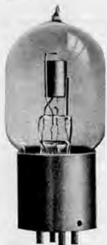
Moorhead Valve, Type SE 1444. Standardized by the United States Government and used by all NC planes in first flight across the Atlantic.
