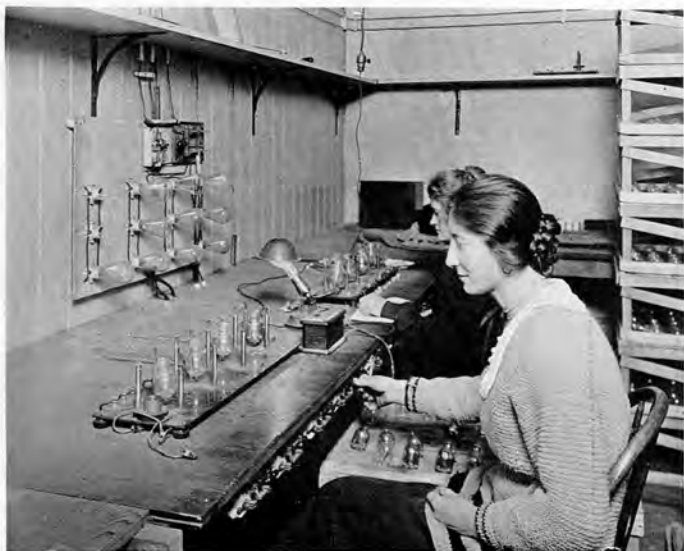
Moorbead Laboratories. Blue glow test after pumping.
