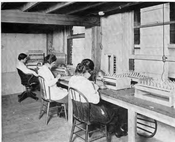
Moorhead Laboratories. Final inspection of assembled elements and attaching filament.
