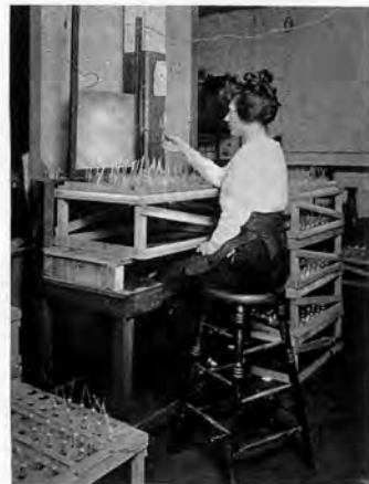
Moorhead Laboratories. Inspecting for defects after sealing.
