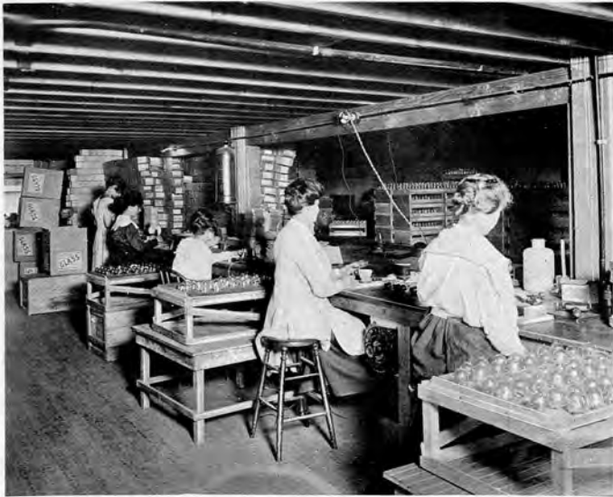
Moorhead Laboratories. Etching and packing valves.
