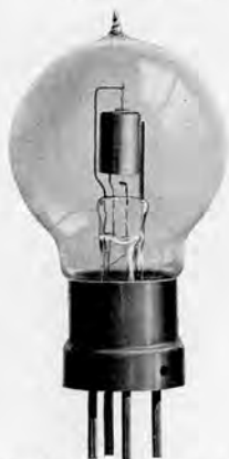
Moorhead Valve. Type R (receiving). Standard of British Government. Used by Allies during the Great War.
