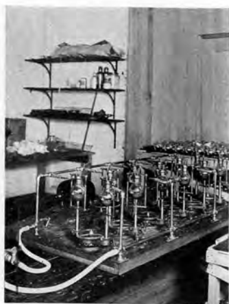
Moorbead Laboratories. Basing machine for cementing brass collars.
