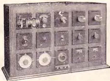
A 15 Panel Cabinet type typical de Forest Unit Receiving Set. Wave length range of tuner 150 to 25,000 meters. Includes a Crystal, Audion Detector and One-Step Amplifier.
