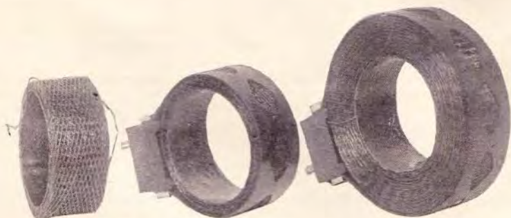
Approximately half size photograph showing open type of winding and relative size of short and long wave coils.
