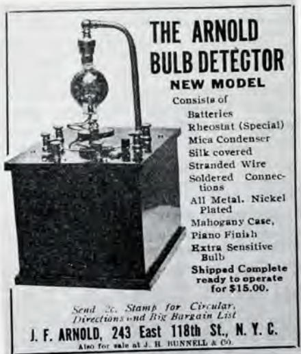
Figure 13 - J. F. Arnold Bulb Detector Reproduced from Modern Electrics, June 1913, page 290.
