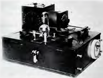
Figure 11 - Wallace Valve Receiver - first form using spherical Audion.
