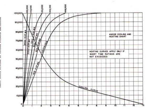
HEAT UNITS STORED IN ANODE DURING EXPOSURE
